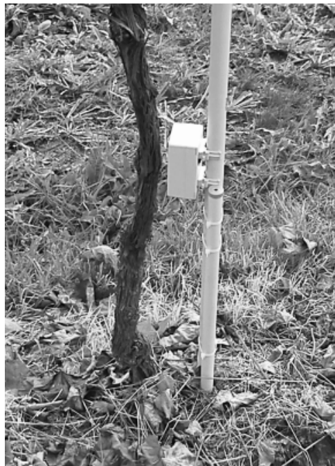
Figure 3. Recording of real-time temperatures driving the S. titanus phenology model. Sensor node at 40cm for recording temperatures relevant for egg development.
