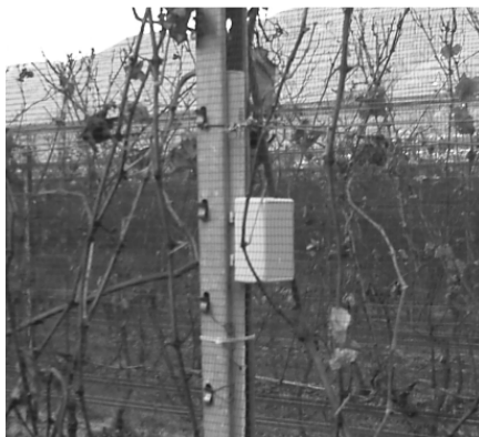
Figure 4. Recording of real-time temperatures driving the S. titanus phenology model. Sensor node at 150cm for recording temperatures relevant for nymph development.
